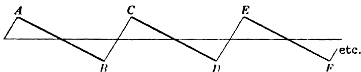
Fig. 38. Trace of the motion of a point on a vibrating violin-string, at a quarter of the string's length from the bridge.
